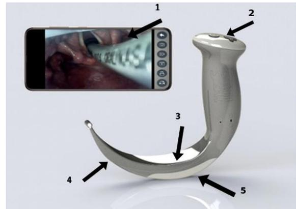
**Figure 1- The SANYAR® Video Laryngoscope: 1) Mobile LCD display; 2) Handle with on / off button and battery charging connection; 3) Blade with a 65° field angle; 4) Camera with an antifog lens; 5) bite lock**
